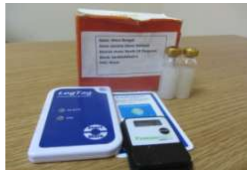
Test box contained, datalogger, un-frozen DPT vials (2) and freeze event indicators (2)
